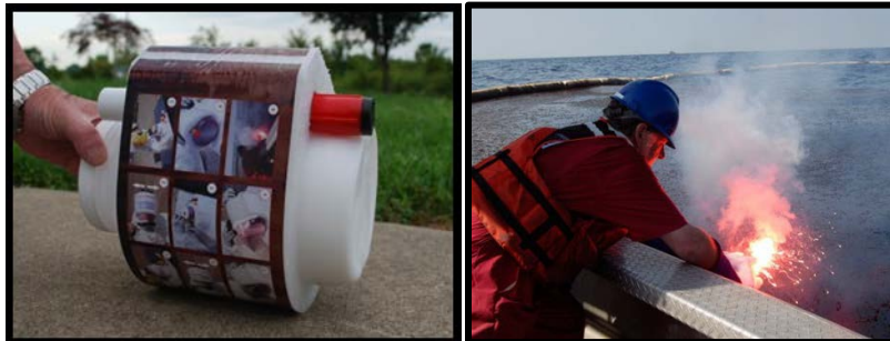
Figure 9407-10: Hand-held Igniter and release upwind of contained oil.
